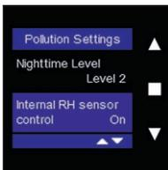
Select the internal RH sensor control using ▲ and ▼, and confirm by tapping ■. You can now use ▲ and ▼ to turn the Endura Delta internal humidity sensor ON or OFF. The humidity sensor is activated as standard, and the Endura Delta will therefore ventilate according to the "pollution triggered ventilation level" if there is an increase in the air humidity (see Daytime Level above).
