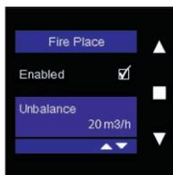
Select “Unbalance” using ■ and change the flow rate using ▲ and ▼. Confirm your choice by tapping ■.
