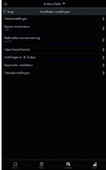
It is important that you, as the installer, configure the flow rates of the ventilation system using this menu in order to guarantee the correct operation of the unit.
