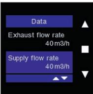
The total supply flow rate for the home is displayed in this bar. This is the sum of all the supply flow rates in your home (all dry rooms). Given that the Endura Delta is a balanced system, the total extraction flow rate is always equal to the total supply flow rate (deviations are possible here when the Fireplace function is active).
