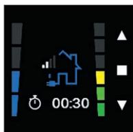
If the timer is active, this is indicated by a stopwatch in the Main menu. In addition, the remaining time is displayed on the timer.
