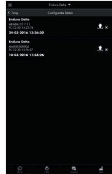
If you tap "Load configuration", then you will see an overview of all the available configuration files. The settings are reactivated by loading one of these files.
