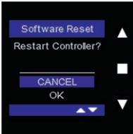
If you wish to continue with the software reset, select "OK" using ▼ and confirm by tapping ■.
