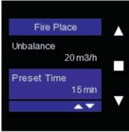
Select "Preset Time" using ■ and change the time interval using ▲ and ▼. Confirm your choice by tapping ■.
