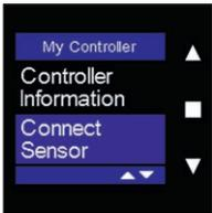
Select "Connect Sensor" using ▲ and ▼, and confirm by tapping ■.
