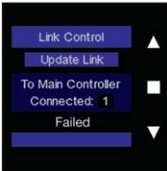
If the link is not made, then “Failed” appears on the screen. Repeat the link procedure.
