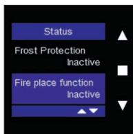
This menu shows you if the “Fireplace function” has been activated or not. The Fireplace function can only be activated using an external switch that can be connected to the 24 V DC input contact on the main board (see 7.1).
