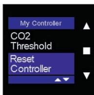
Select "Reset Controller" on the Main/Sensor Controller using ▲ and ▼, and confirm by tapping ■.
