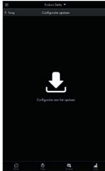
If you tap "Save configuration", then a copy is made of all the settings. This copy can be loaded later.
