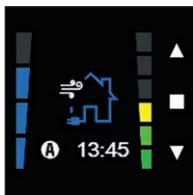
The main screen will now display a house with wind blowing to indicate that the Breeze timer is activated. In addition, the remaining time is displayed at the bottom of the timer.
