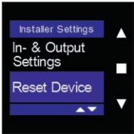
Select "Reset Device" using ▲ and ▼ and confirm by tapping ■.
