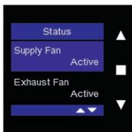
This menu displays the status for the supply fan. If “Active” is displayed, then the supply fan has been activated. If “Inactive” is displayed, then the supply fan has been deactivated and you must check to see if an error message has appeared in the Error Log (see Section 8.1.3.4.1.8).
