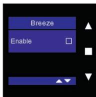
You can activate the automatic “Breeze function” and set the parameters for this function using this menu. The Breeze function is used to actively cool down the home during warm summer months. The Bypass valve closes the heat exchanger so that the supplied air is blown into the home unheated in order to cool the home down.
