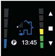
After confirming your country, the Main Controller menu opens. You can now begin correctly programming the Endura Delta. Use the Installer menu "Settings > Installer settings > Flow rate settings" for this. See Section 8.2.3.1.
