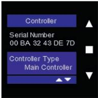
You can find out whether the controller is set as the "Main Controller" or as the "Sensor Controller" air quality sensor here.
