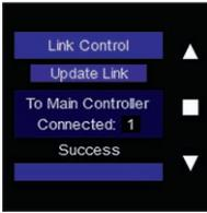
Once the link is successful, “Success” appears at the bottom of the screen and the main screen opens.
