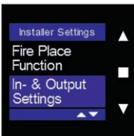
Select "In- & Output Settings" using ▲ and ▼, and confirm by tapping ■.
