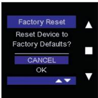
Select "OK" using ▼ and confirm by tapping ■ to delete the current settings and reset them to the factory settings.
