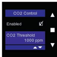
In order to change the threshold, select “CO<sub>2</sub> Threshold” using ▲ and ▼, and confirm by tapping ■.
