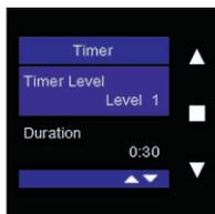
You can change the timer level by first briefly tapping ■. Use ▲ and ▼ to select a timer level, and confirm your choice by tapping ■. As soon as you start the timer, the ventilation system will start ventilating at the selected level.
