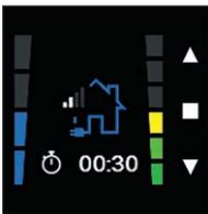
By tapping ▲ in the main screen, you can temporarily move from Level 1 (automatic mode) to Level 2 (manual mode).
