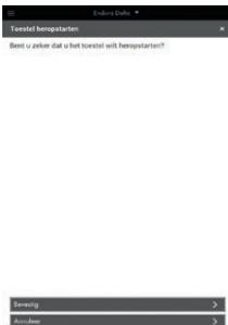
"Restart device" is not the same as "reset device" (see 10.2.5.1.14). "Restart" means that only the unit is restarted. No settings will be deleted. "Reset device" means that all of the settings are deleted and the default factory settings will be restored.
