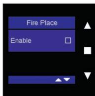
Tap ■ to activate the function. The Fireplace function can only be controlled via an external switch! (See Section 7.1 for the electrical diagram.)
