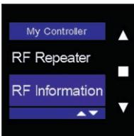
Select "RF Information" on the Sensor Controller using ▲ and ▼, and confirm by tapping ■.
