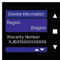
You can change the regional settings using this menu. Every country has a specific configuration for the unit based on the applicable ventilation requirements.
