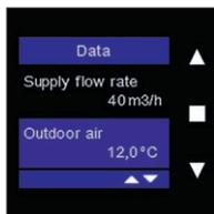
This bar displays the temperature of the outdoor air that is being blown into the home. This is the temperature of the outdoor air before it is heated in the heat exchanger.
