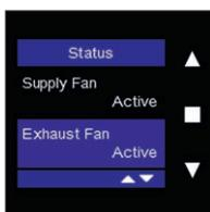
This menu displays the status for the extraction fan. If “Active” is displayed, then the extraction fan has been activated. If “Inactive” is displayed, then the exhaust fan has been deactivated and you must check to see if an error message has appeared in the Error Log (see Section 8.1.3.4.1.8).
