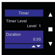
You can set the time intervals for the timer in the “duration” by first briefly tapping ■ and then using ▲ and ▼ to change the time in 5-minute intervals. The maximum time for a timer is 8 hours. The minimum time is 5 minutes.
