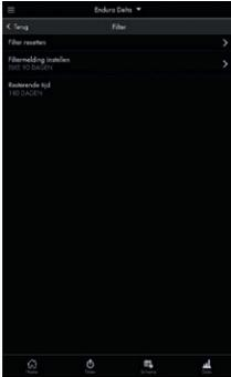
You can use this menu to reset the filter time, set the filter time, and see how many days are left until you must clean/replace the filters. We recommend cleaning the filters every 90 days and replacing them every 180 days.
