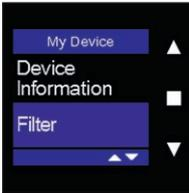
Select "Filter" using ▲ and ▼, and confirm by tapping ■.
