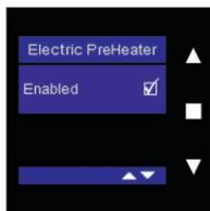
The electric preheater is enabled by default if the Endura Delta is equipped with an electric preheater. To turn off this function, briefly tap ■.
