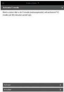
You can activate the "C-mode" (design position) using this menu. If the C-mode is active, then the Endura Delta will nominally ventilate for 30 minutes. You can calibrate the system during this half hour by adjusting the supply and extraction valves. The flow rates must be verified when the C-mode is activated.
