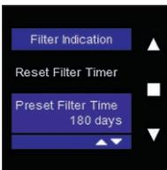
You can set the time for the filter timer using this menu. You can choose to get a message every 90, 180, 270, or 360 days when it is time to clean/replace the filters.
