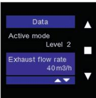
The total exhaust flow rate for the home is displayed in this bar. This is the sum of all the extraction flow rates in your home (all wet rooms). Given that the Endura Delta is a balanced system, the total extraction flow rate is always equal to the total supply flow rate (deviations are possible here when the Fireplace function is active).
