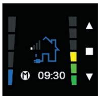
An M is displayed at the bottom left of the TouchDisplay as long as the manual mode is active on the XVK 4-position switch.
