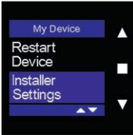
Select "Installer Settings" using ▲ and ▼, and confirm by tapping ■.
