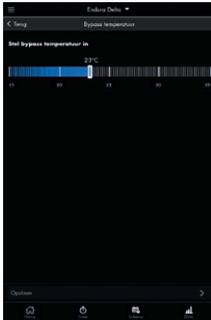
You can change the Bypass temperature using this menu. This is set to 23°C (indoor temperature) by default. The Bypass is activated when the following conditions have been met:
