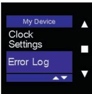
Select "Error Log" using ▲ and ▼, and confirm by tapping ■.
