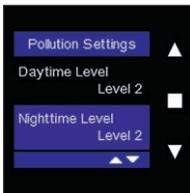
Select "Nighttime Level" using ▲ and ▼, and confirm by tapping ■. You can now use ▲ and ▼ to change the ventilation level for the demand side for the night period. Confirm your choice by tapping ■.
