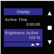
Select "Brightness Active" using ▲ and ▼, and confirm by tapping ■.
