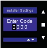
Change the code using ▲ and ▼, and confirm each time by tapping ■. To exit the menu, briefly tap ▲ and ▼ simultaneously.
