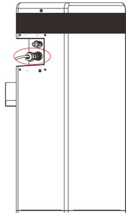
2. Insert the other end of the CAN communication cable to the CAN connector (II) on the first battery which is marked in red. Assemble the cable gland and tighten the cable cap.
