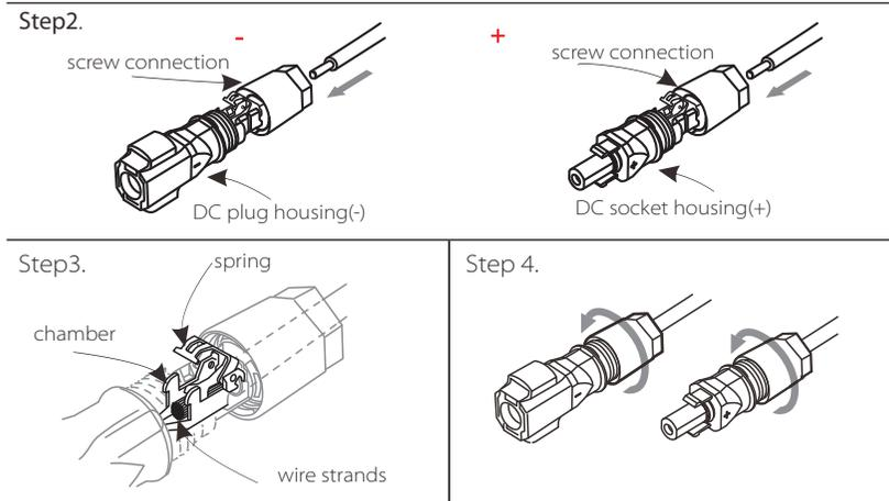
➤ Connecting Charging Cables between Inverter and T-BAT System:
