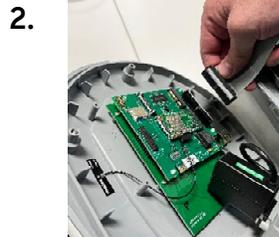
2. Unscrew the cover and unclip flat ribbon cable.
