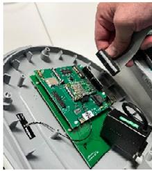
Re-fit the cover ensuring the ribbon cable is seated firmly, both in the zappi and onto the back of the cover.
