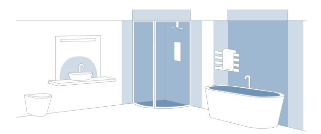
When installing Waves in the bathroom, you have to take into account that the bathroom is divided into 4 zones (0-3). Based on the IP class, the device can be placed in zones 2 or 3.
